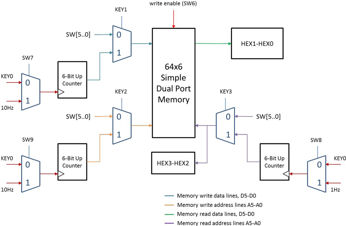
Input data for writing to the memory is to be selectable (using KEY1) from either SW[5..0] or from a 6-bit up counter. The 6-bit data up counter is to be clocked from KEY0 or from a 10 Hz clock source (using SW7 to select the clock source). An input address for selecting a memory location to write is to be selectable (using
